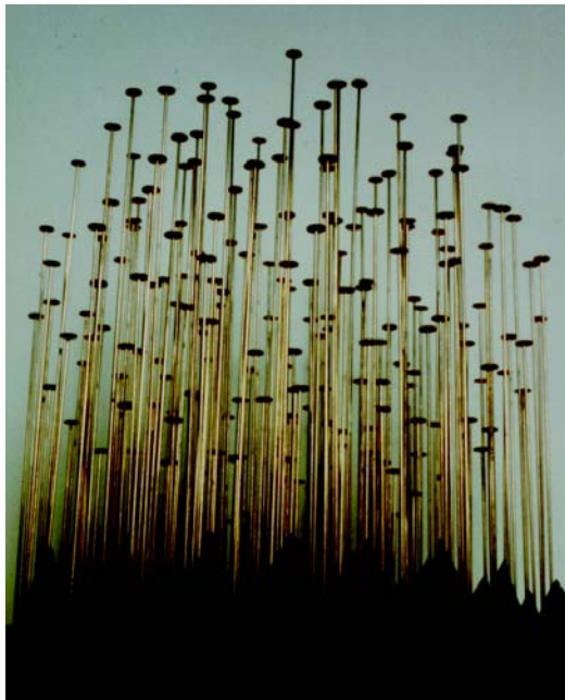
(a) Crow's Nest antenna with 512 elements randomly distributed
